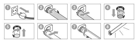
The LED replacement starter in the package is mandatory for operation and safety
