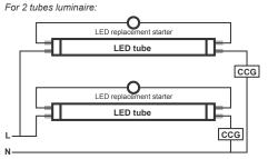
LED tube only suit parallel mounted ballast. In case a parallel power factor compensation capacitor is used in the luminaire, it will reduce the power factor. Consider that power factor could need to be adjusted according to local regulations.
